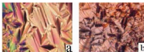
Figure 1. Microphotographs obtained in between the crossed polars: (a) focal conic fan-shaped texture of smectic-A (Lamellar) phase (250X) (b) focal conic fans with radial striation of smectic-E phase (250X).
